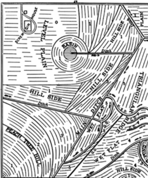
Figure 7.--Sorsby's plan for diversified erosion control on a 45 acre plot: 0, Straight rows run by the eye; 1, level culture; 2, level culture with guard drains; 3, grading method No. 1; 4, grading method No. 2; 5, grading method No. 3.
